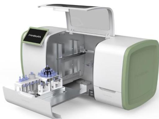
The PANBioRA prototype: cytotoxicity test loading
